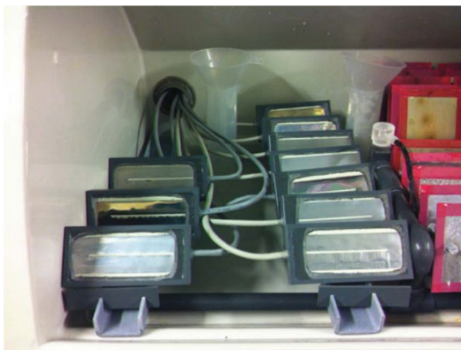
Figure 2 - Probes (L) before and (R) during testing in the salt spray chamber according to ASTM B117.
