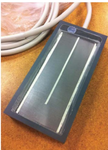
Figure 2 - Probes (L) before and (R) during testing in the salt spray chamber according to ASTM B117.
